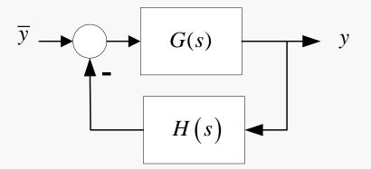
The closed loop input response transfer function is
